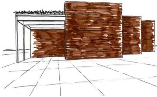
The walls carry the loads from the timber roof above. To ensure the durability of the structure, the roof is designed to overhang most of the walls and protect them from the rain. The elements of exposed wall are protected by adding cement to the basic soil mix.
